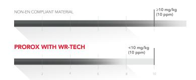
\*ROCKWOOL Technical Insulation has developed WR-Tech, an advanced water repellency technology based on a unique binder that repels water and has a low chloride content.
